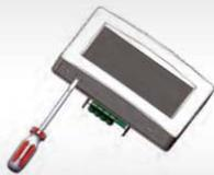
Carefully separate the front half of the thermostat from the back plate by placing a small flat head terminal driver into the slots on the bottom face of the thermostat.
